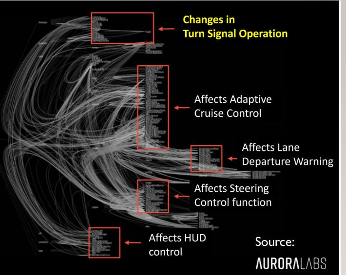
Impact of a recoding for changes in turn signal can impact multiple functions
